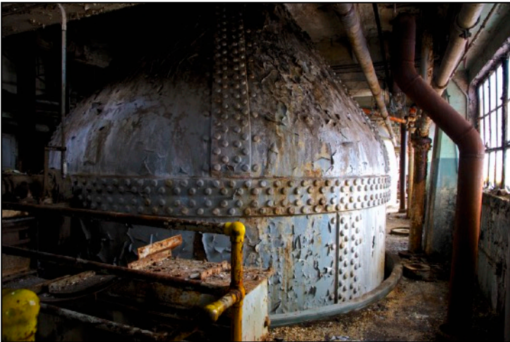
Midway up West Linn Paper’s towering Mill B, is the top of the five, multi-story digesters that were used in the sulfite process for making pulp.
