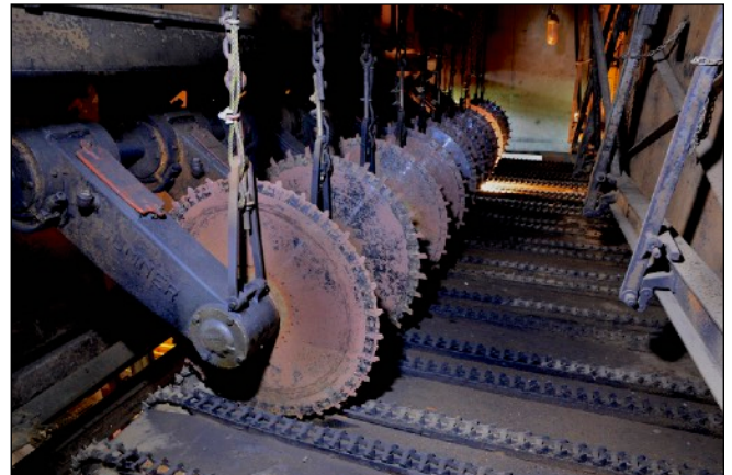
A gang of slasher saws used for trimming cants down to 24" blocks that could be manually handled.
