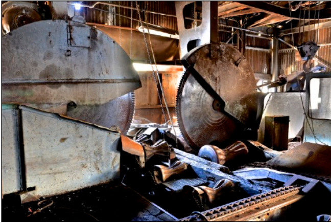
Upon entering the mill, logs were cut down to a manageable length by these massive circular saws.
